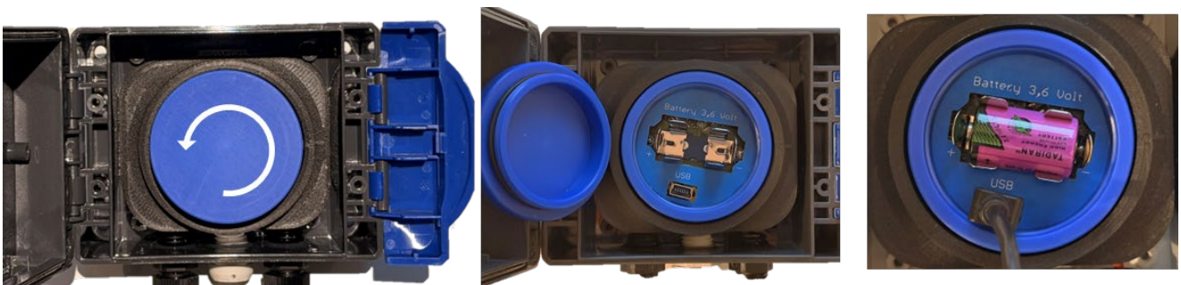
Figure 5- A round data logger is seen once the unit is opened. Unscrew the lid gently and place the battery in.
