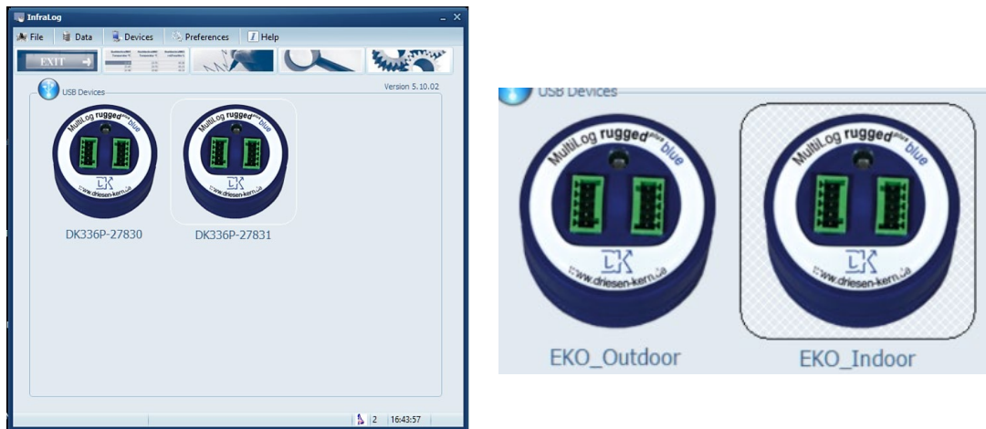
Figure 6- Initial look of the software (left). Click on the logger images to see the names (right)
