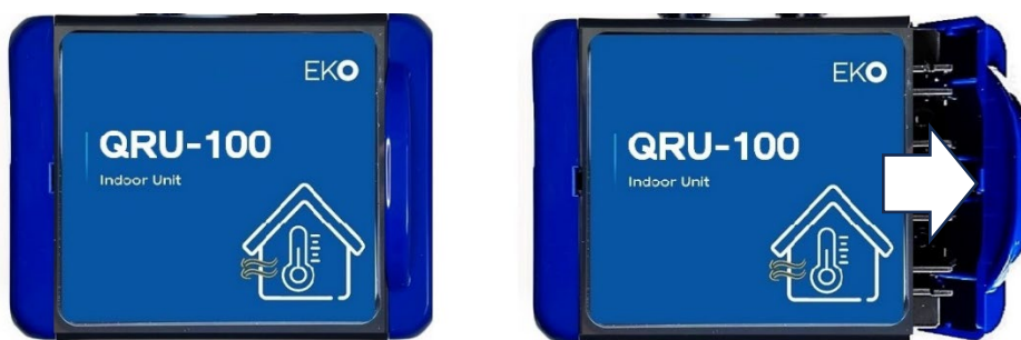
Figure 4- Press the blue handle to open the lid of the Indoor Unit.
