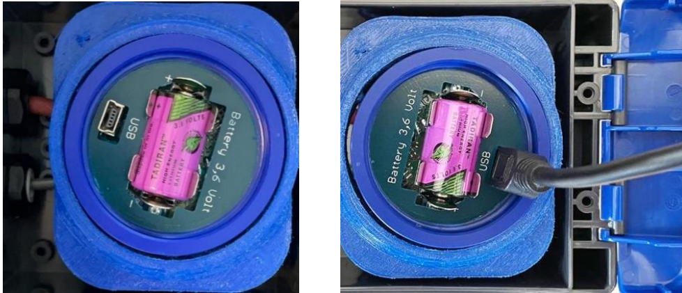
Figure 3- A round logger can be observed once the unit is opened. Locate the USB port and connect the unit to the PC using the USB port.
